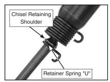
Figure 4. Safe chisel position.
